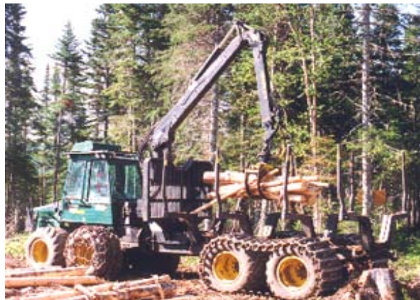
Figure 7-4. Rubber-tired forwarder transports the 2.50-metre bolts to roadside.
